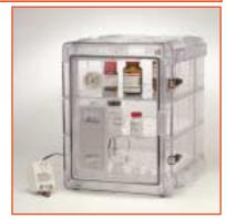
for different contents. The door opening is 31.2H X 22.5cm W (12.3H X 8.9"W) and includes 2 latches and loops for lock or tamper evident seal. Shipping weight 10 Kg (22 lb.).
